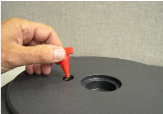
Figure 8: Remove red plug before loading
